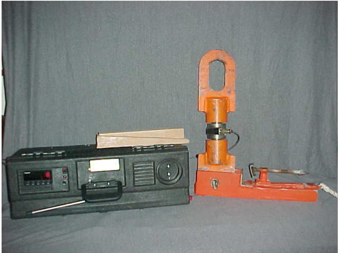
The loadcell pictured above has a capacity of 50,000 lb.
