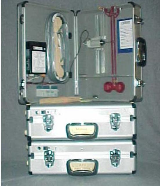
The Pendulum Arm is balanced on two adjustable pivots that are honed to a point about the same size & shape as a fine ballpoint pen. The pivots are vertical and parallel to the arm. The weight is 32 oz. The couple between the Arm & the Transducer Rod is magnetic for no friction resistance. The rod has 10 grams of resistance.
