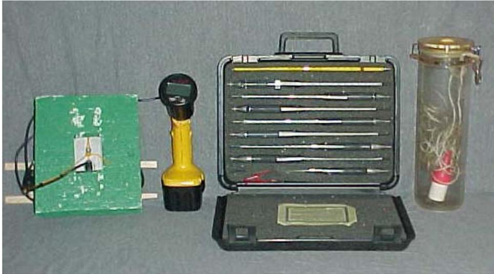
Depth Soundings are taken at the same locations as the Freeboard Readings and recorded on the Incline sheet. The green unit pictured above is a float with the Sonar unit mounted at center. The unit with readout is hand held and is a HAWK EYE Sonar unit Model: DF1000D with readouts at 1/10 of a foot.
