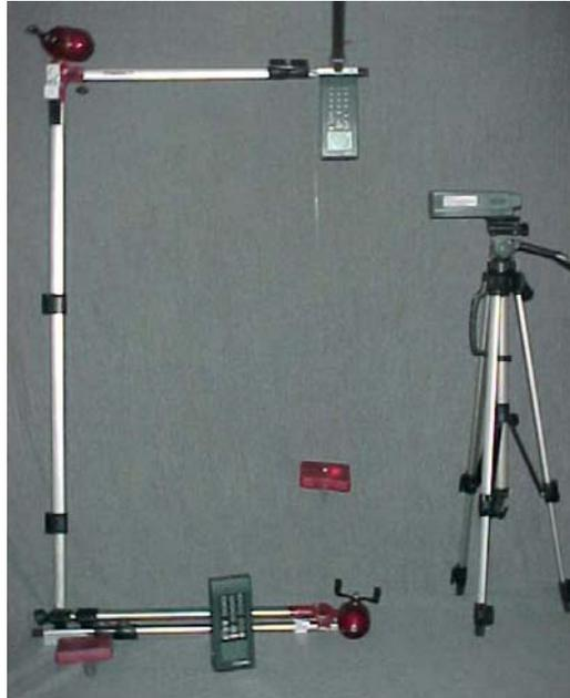
Freeboard measurements are accomplished by the use of Disto Pro 4a laser measuring devices on stands as pictured above left. The stand base is set on deck at sheer, the line plumbbob with float is lowered into the water and the unit is turned on. The operator then aligns the laser dot on the float as pictured and takes a reading with a press of a button. This reading is automatically sent to the Laptop for recording. This reading is from sheer to water with all offsets done by the Disto unit.
