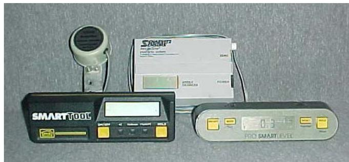
The Trim of the vessel during the Incline is monitored by the use of any one of the above-pictured electronic levels. The two levels pictured in the foreground read to 0.0° and have no certifications but have been found to be accurate. The Accu-Star Protractor pictured in the background reads to 0.00° and has NIST traceable certifications. There is no ASTM standard set for this equipments application in Incline Tests.
